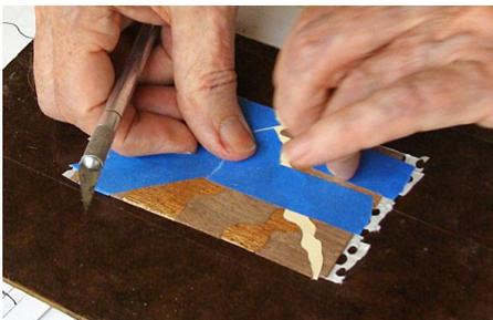
After removing the panel from the caul plates, **Chris** flipped the veneer panel over to expose the bottom side with the painter's tape. This is the side of the panel that will ultimately be glued to the substrate. All of the strips of painter's tape were carefully removed so as not to misalign any of the veneer pieces.
