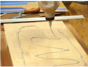
He then applied **Titebond Cold Press Veneer Glue** to his plywood substrate. One person suggested that as a rule of thumb, approximately 1 ounce of glue per square foot of substrate provides sufficient bonding in most cases. Though other glues can be used successfully as well, this **Titebond Cold Press Glue** product probably has an extended open time to aid assembly of a veneered panel.
