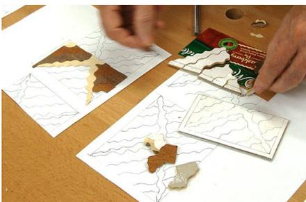
And now the fun begins! Carefully separating individual pieces of veneer from the cut stack, **Chris** began assembling them onto the previously printed patterns. These pieces were placed **with the best side down** against the pattern in accordance with his predetermined set of panel layouts to produce the desired species, color, and grain pattern mix.
