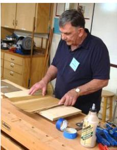
Then he selected his pieces of veneer, carefully orienting the pieces to produce the most pleasing grain pattern, deciding where to trim the pieces to suit the panel requirements and remove some of the unwanted defects and sapwood areas.
