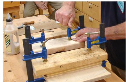
**Herb** also used clamp blocks on top of the **upper caul plate** to improve the uniformity of the force application from the clamps. He noted that the clamps and clamp blocks must be applied to the **center of the panel first**, with the outer ones applied sequentially, working toward the outer ends of the panel. This technique tends to squeeze any excess glue from the center of the panel toward the outer ends. He also noted that “More and heftier clamps are better!”
