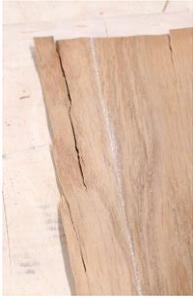
**Herb** noted that veneers commonly have splits and other defects near the ends of the pieces due to the brittle nature of the material. However, many of these imperfections can be overcome by simply pulling them together and securing them with a strip of tape. He used that technique in several places on his demonstration panel
