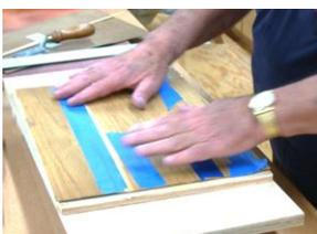
He then applied the veneer panel to the glue-covered substrate and smoothed it with his hands, noting that some folks roll the surface to produce intimate contact and even out any excess glue.
