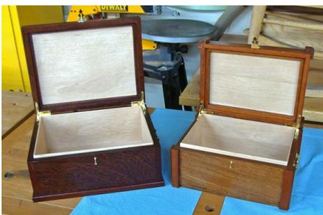
**Herb** noted that both of the humidors employed a similar construction method – veneered panels with abutting solid wood corner posts. He said that was an effective way to cover the exposed ends of the box panels and veneers. It also seemed as though this construction technique added to the appearance of solid sturdiness to the humidors. Well done, **Herb!**
