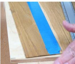
He then butted the two veneer strips tightly together and applied a strip of painter's tape to the full length of the joint. He noted that paper veneer tape, either solid or perforated, is also commonly used to secure the
