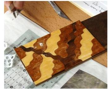
The final operation was the sanding of the veneered panel. **Chris** noted that a random orbit sander (ROS) works well for this task, starting with 120 grit disks if the surface is uneven and 220 grit if the surface is fairly even. He cautioned that the ROS tends to thin the edges of the panel, so it is wise to make the panel oversize, allowing final trimming to remove any thinned edges.
